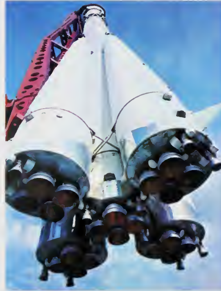
Soviet launch vehicle used to place manned Vostok spacecraft into orbit. Based on the R-7 intercontinental ballistic missile, the launcher had four strap-on liquid-fuel boosters surrounding the liquid-fuel core rocket.
